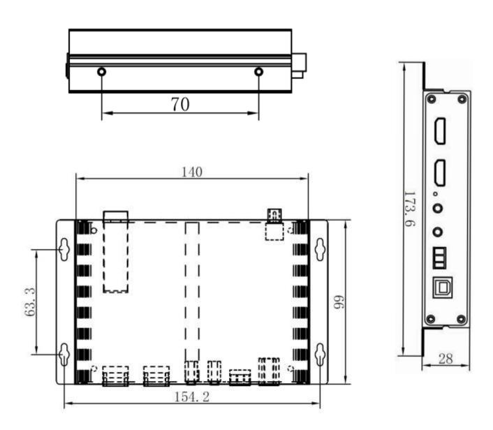
The VOS-1HDMI-ADT transmitter/VOS-1HDMI-ADR receiver can be installed into our rack mount chassis, VOS-CH04, which can be mounted into an industry-standard 19-inch equipment rack.
