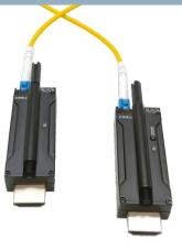
The Fiber Extender support HDMI 2.0, resolution up to 4K 60Hz (4:2:0), 4K 30Hz (4:4:4), Backward compatible. EDID is managed by maintaining continuous EDID communication with the source, ensuring that it powers up properly and maintains video output. For HDMI signals with protected content, the VOS-HDMI-T/R-Mini continuously authenticates HDCP compliance to support quick and reliable transmission, desinged to solve the installers common problems with long distance HDMI transmission.
