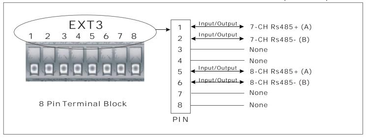
Receiver (RS485): 8-Ch 2-wire Rs485 Data (In/Out)
