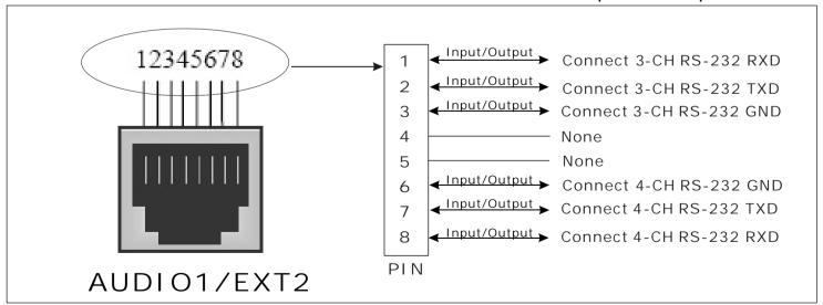
Receiver (Rs232 Data): 8-Channel Duplex Rs232 Data Connection (Input/Output)
