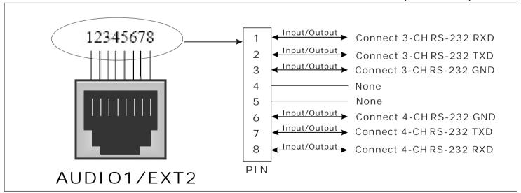
Transmitter (Rs232 Data): 8-Channel Duplex Rs232 Data Connection (Input/Output)
