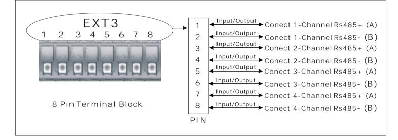
Receiver (Rs485): 4-channel duplex Rs485 Data Connection (Input/Output)
