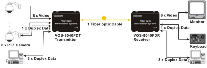
NOTE1: Digital video optic transmitter and receiver should be used in pairs, one is Transmitter (LED is red), the other is Receiver (LED is green).
