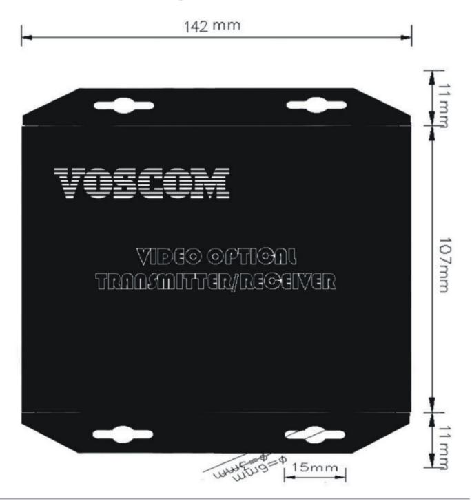
The VOS-4FOM-D232T transmitter/VOS-4FOM-D232R receiver can be installed into our rack mount chassis, VOS-CH04 or VOS-CH06, which can be mounted into an industry-standard 19-inch equipment rack.
