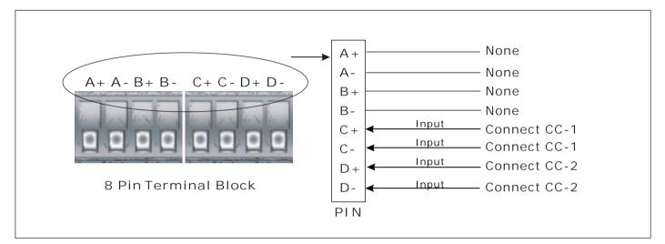
Receiver: 2-Channel Simplex Contact Closure Connection (Output)
