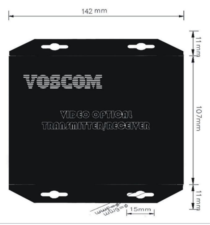
The VOS-2FOM-SCCT transmitter/VOS-2FOM-SCCR receiver can be installed into our rack mount chassis, VOS-CH04 or VOS-CH06, which can be mounted into an industry-standard 19-inch equipment rack.
