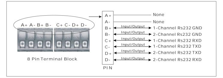
Receiver: 2-Channel Duplex Rs232 Data Connection (Input/Output)
