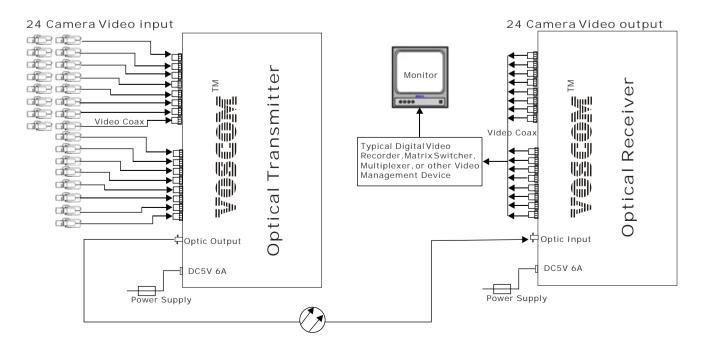
The VOS-24000FT transmitter/VOS-24000FR receiver only support Stand-alone 19 inch 2U rack. All units of VOS-24000FT/R can not be used by video card style.
