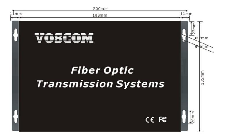
The VOS-1VGA-LT transmitter/VOS-1VGA-LR receiver can be installed into our rack mount chassis, VOS-CH04-HD16 which can be mounted into an industry-standard 19-inch equipment rack.
