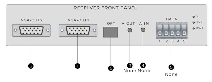
**1** VGA-OUT1 HD-15 VGA Connector: The first channel VGA output.
