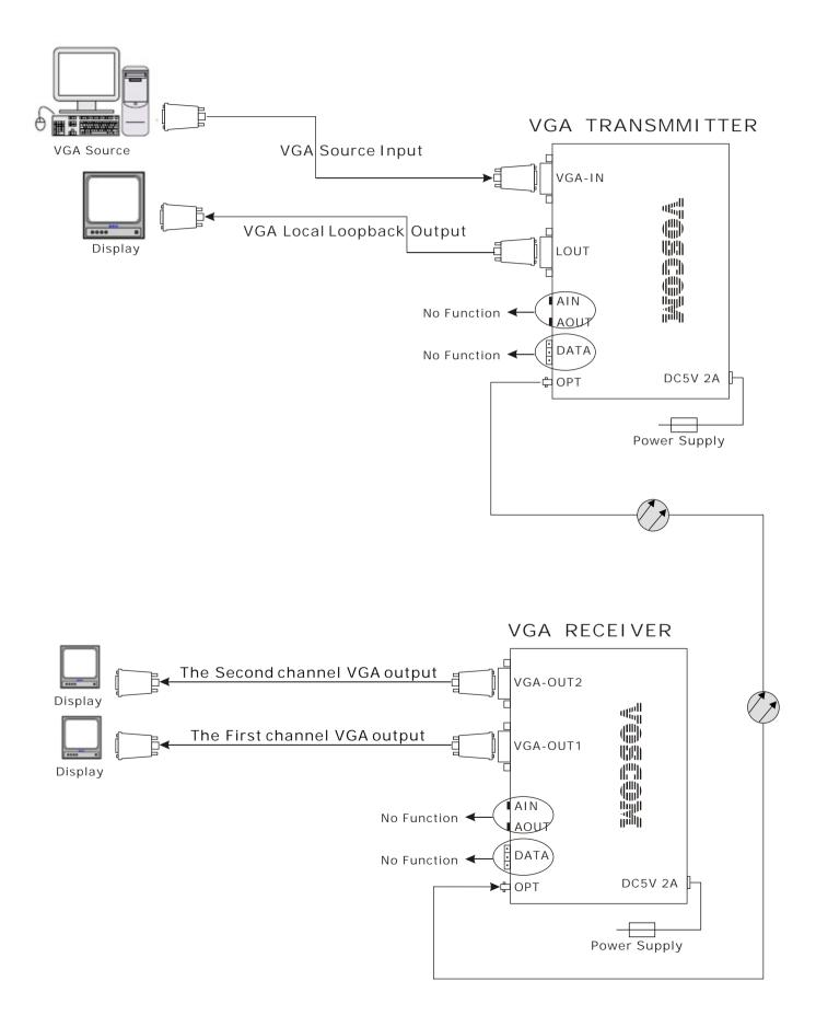
The VOS-1VGA-LT transmitter/VOS-1VGA-LR receiver can be mounted into a rack or can be used as a stand-alone module. As a stand-alone module, the unit can be placed on a desktop or can be mounted to a wall.
