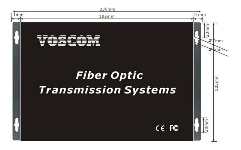
The VOS-1HD-T transmitter/VOS-1HD-R receiver can be installed into our rack mount chassis, VOS-CH04-HD16 which can be mounted into an industry-standard 19-inch equipment rack.
