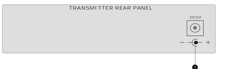
Stand-alone Power supply Connector: DC5V 2A Input
