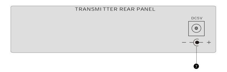
Stand-alone Power supply Connector: DC5V 2A Input
