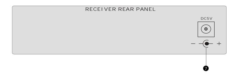
7 Stand-alone Power supply Connector: DC5V 2A Input
