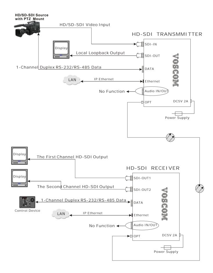
The VOS-1HD-DET transmitter/VOS-1HD-DER receiver can be mounted into a rack or can be used as a stand-alone module. As a stand-alone module, the unit can be placed on a desktop or can be mounted to a wall.
