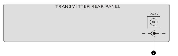
Stand-alone Power supply Connector: DC5V 2A Input
