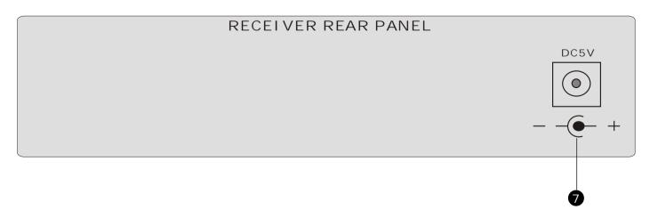
Stand-alone Power supply Connector: DC5V 2A Input
