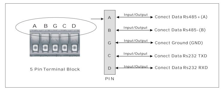
Receiver (Data): 1-Channel Duplex Rs232/Rs485 Data (Input/Output)
