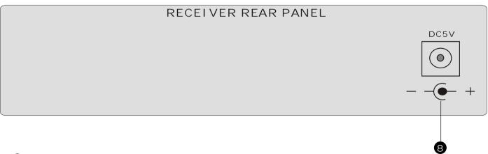
Stand-alone Power supply Connector: DC5V 2A Input
