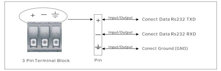
Receiver (Rs232): One Duplex Rs232 Data Connection (Input/Output)
