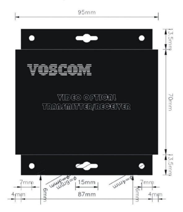
The VOS-1FOM-D232T transmitter/VOS-1FOM-D232R receiver can be installed into our rack mount chassis, VOS-CH04 or VOS-CH06, which can be mounted into an industry-standard 19-inch equipment rack.
