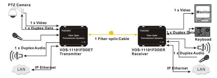
NOTE1: Digital video optic transmitter and receiver should be used in pairs, one is Transmitter (LED is red), the other is Receiver (LED is green).
