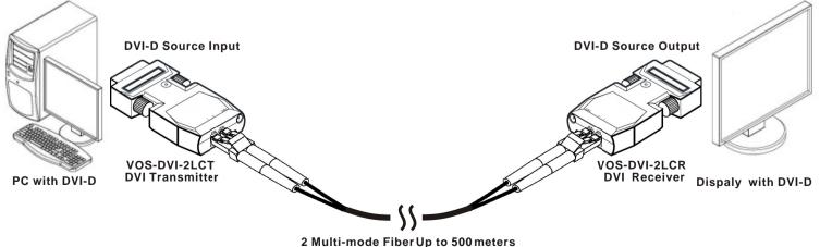
2 Multi-mode Fiber Up to 500 meters 2 Single-mode Fiber Up to 1500 meters
